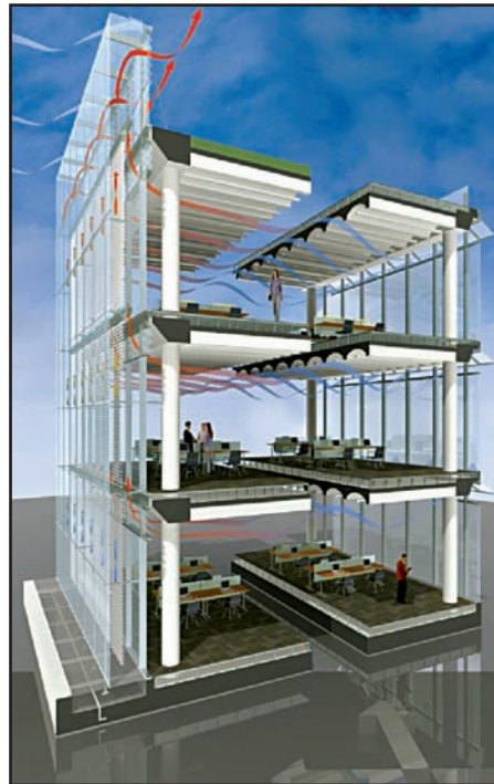
FIGURE 2. Computational flow dynamics was used to design Klarchek Information Commons at Loyola University Chicago.
