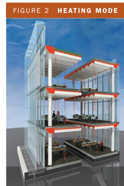
When the building is in heating mode (designed to operate 202 days per year), the ceiling provides radiant heat to the space with supplemental convection finned tube on the east side only.
