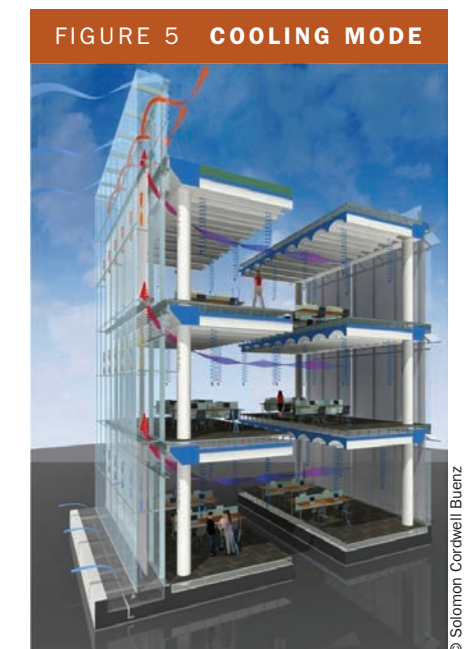
In cooling mode (designed to operate 50 days per year), a ducted underfloor air system provides ventilation air and supplements the radiant ceiling cooling system on design days.
