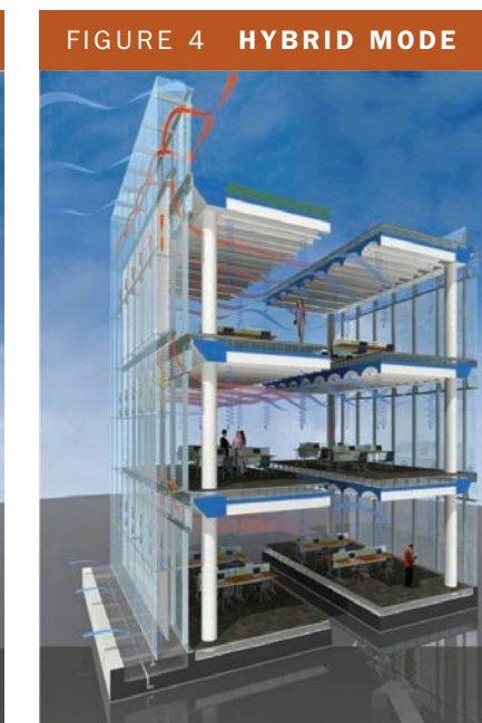
In the hybrid mode (designed to operate 62 days per year), windows are open, all fans are off, and the ceiling is chilled to provide radiant cooling. This mode allows natural ventilation to occur at higher outdoor air temperatures.
