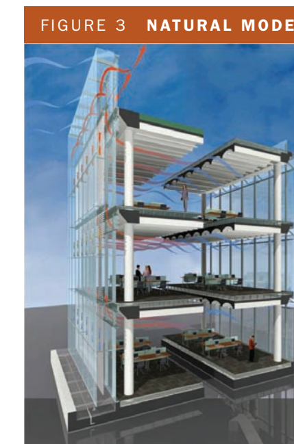
In natural ventilation mode (designed to operate 52 days per year), automatically controlled operable windows on the east façade and the inner windows on the west double façade are opened.
