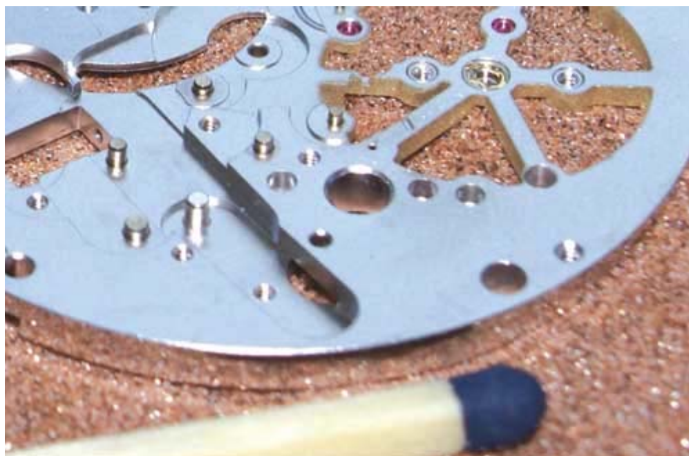
Cuts were made in this watch base plate after the rubies went in.
